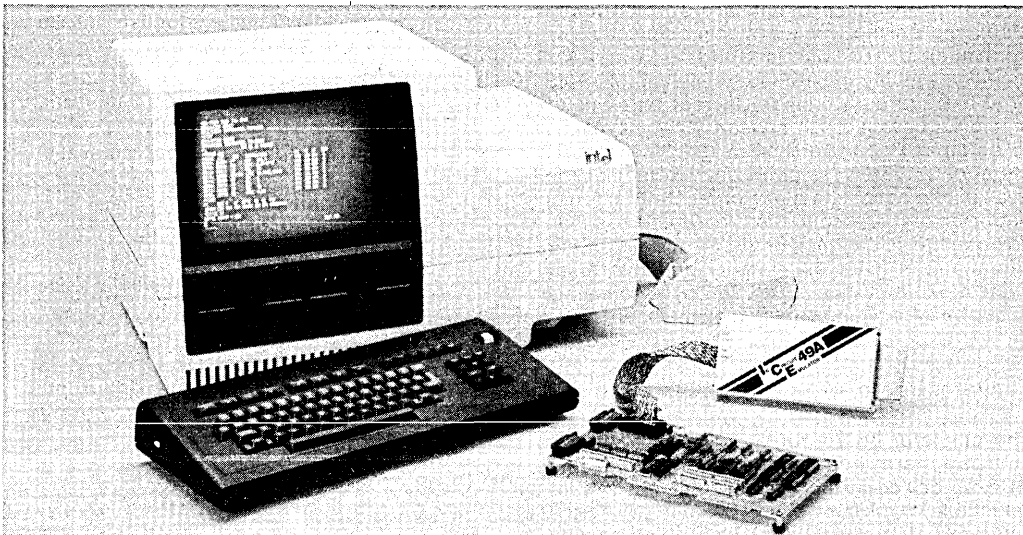
Figure 2. The ICE-49A module hosted by a Series IV development system and connected to a user prototype board.
